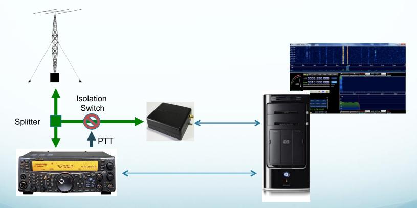
DO NOT directly connect the RSP to the same antenna as your transmitter as this is likely to result in irreversible damage to your RSP and invalidate your warranty. www.sdrplay.com
