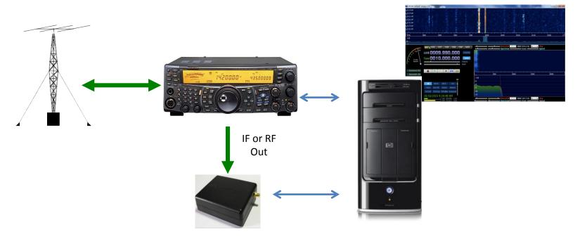
IF Out: - Displayed bandwidth limited by transceiver on-board filters
