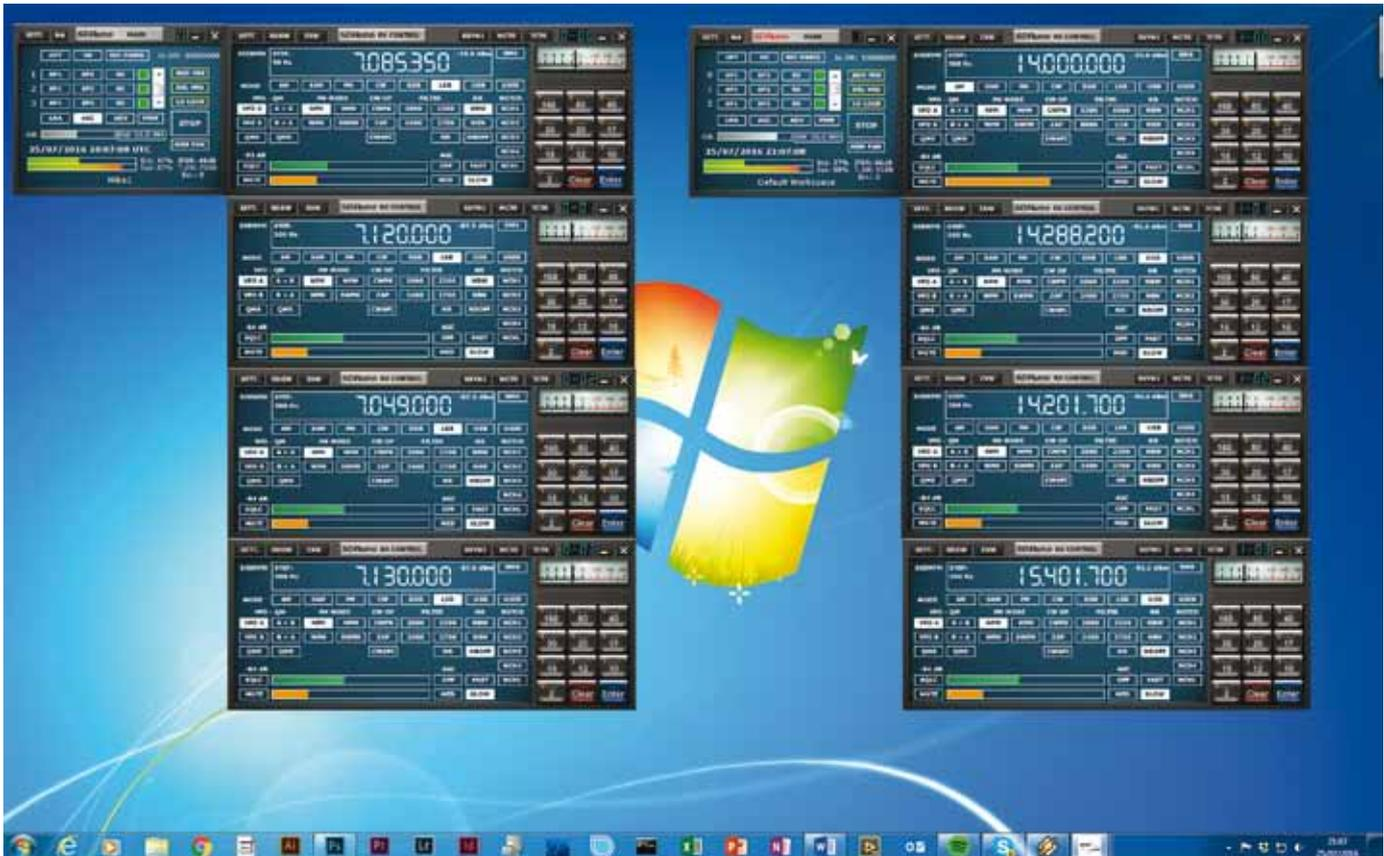
Fig. 8: SDRUno with two instances and 8 receivers running on an Intel Core i5 quad-core PC.
