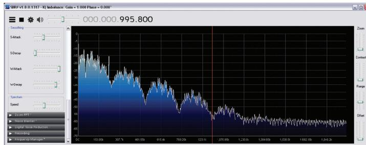
**PHOTO 1:** The SDR-Play module used with the *SDR#* software as a spectrum analyser. Here is it showing the spectrum of the spread spectrum source of Figure 1, with a chip rate of 250kHz.
