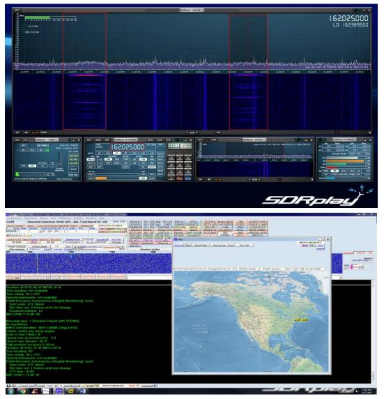
You will need either VB-Cable or VAC installed and configured. This will allow you to pipe the audio out of SDRuno into the MultiPSK decoder.
