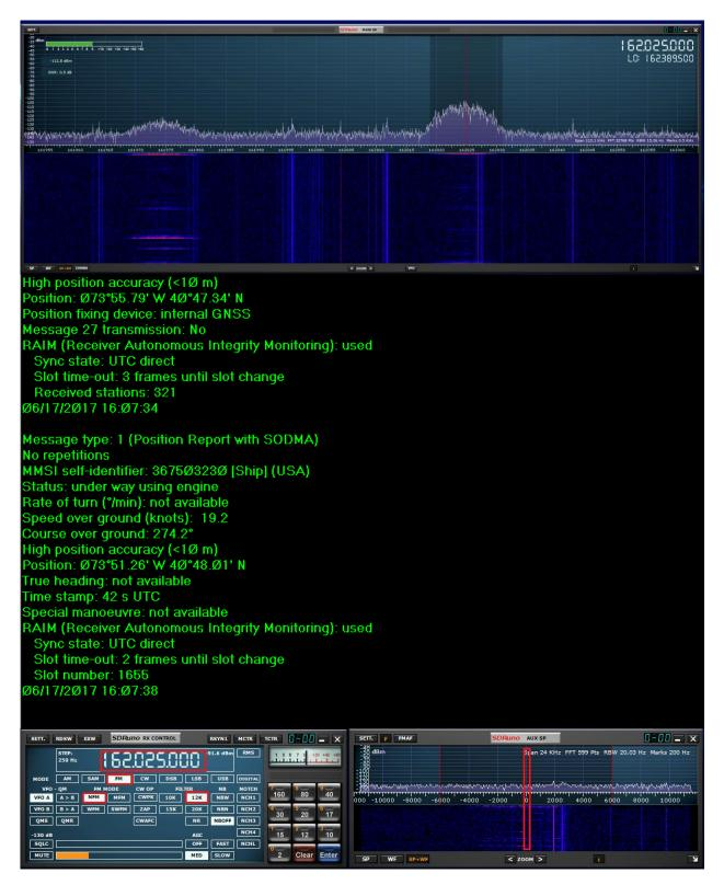
\* Center the peak of the AIS burst as shown in the AUX SP Module
