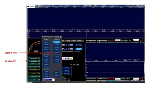
The HDSDR *bandwidth* button controls output sampling rate. The default setting is 12,000Hz. For WFM (wide band FM) you need to move this to 192000Hz
