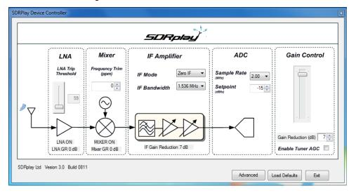
**LNA Trip Threshold** – The point at which the LNA turns on/off within the gain reduction range can be controlled by value in the LNA Trip Threshold. By lowering the value the LNA will turn off closer to maximum gain. Increasing the value means that the LNA will stay on for longer thus providing better noise performance but at the added risk of overload.
