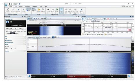
Figure 9 — In addition to decoding FM stereo, SDR Console decodes the RDS (Radio Data System) text streams.
