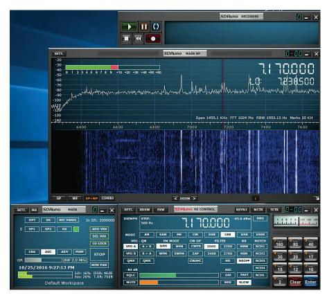
Figure 7 — RSP1 receiving on 40-meter SSB using *SDRuno* software. Only one receiver is shown here, but the application can open several simultaneously.
