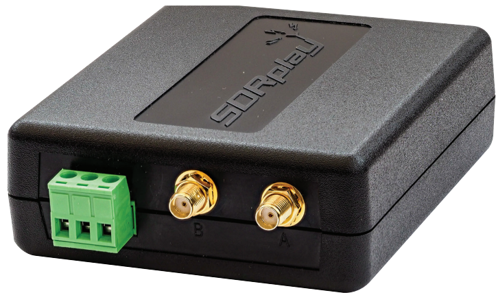
PHOTO 1: SDRplay RSP-2 general view. The two SMA sockets are the main antenna connections and the green block is a detachable high impedance (1000Ω) input.
