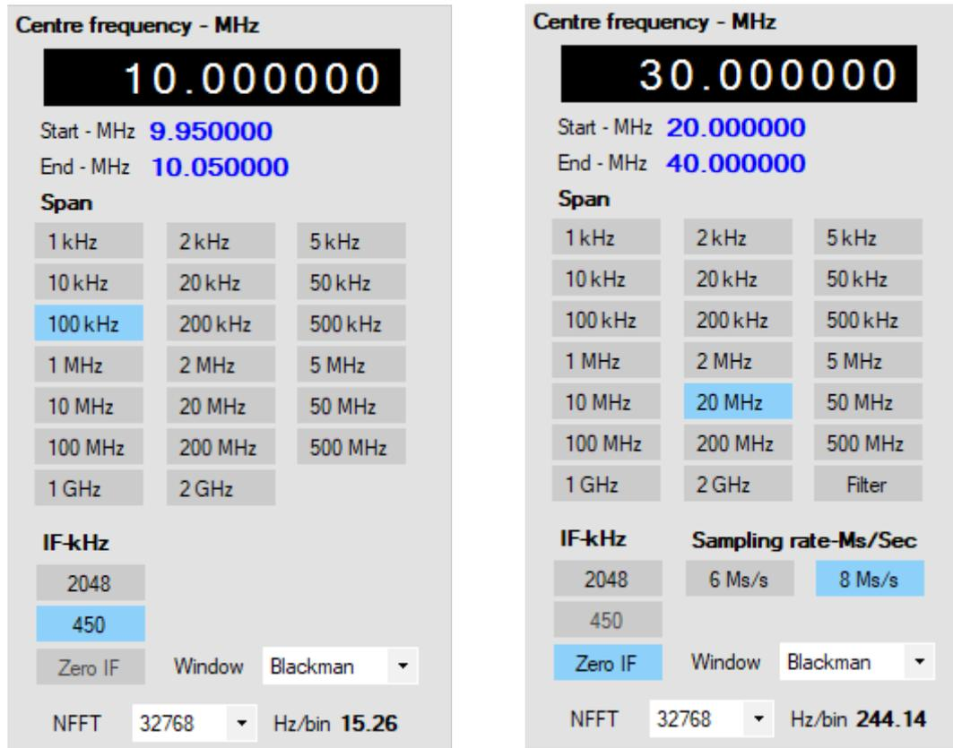
**Centre freq** is used to set the centre frequency of the current span. There are two ways of entering or changing the centre frequency.
