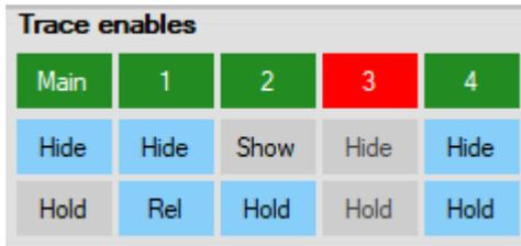
The trace enables panel controls the enabling, displaying and holding/pausing of each trace. There are five available traces. The Main trace has the same properties as any of the other traces.
