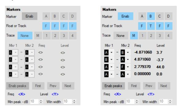
The marker control panel handles the allocation of four markers A, B, C and D. Each marker may be allocated to one of the five available traces, provided the trace is enabled. In addition, the panel controls the peak find functions and marker mathematics.
