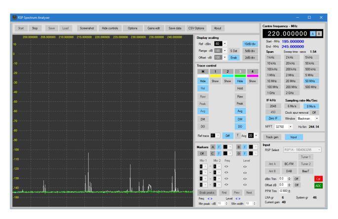
Apply the average offset by clicking on **DO**. The trace should now be plotted at the average level of the reference trace.
