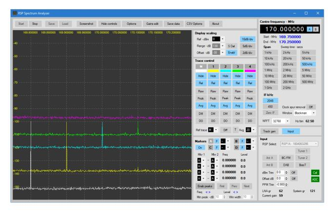
This clearly shows that setting the reference level to a higher level (towards 0dBm) increases the noise floor and reduces sensitivity. At a reference level of -20dBm the S/N ratio has been reduced to 10dB, and at 0dBm reference, the signal is around 3dB below the noise floor and is not detected.
