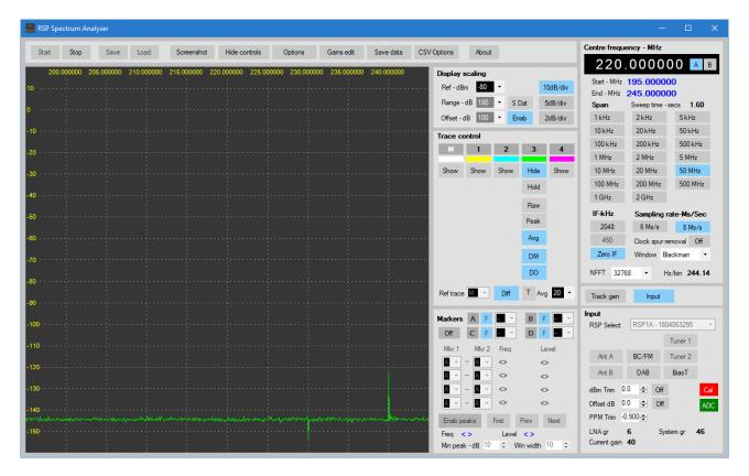
The frequency is now changed to 240MHz. Note the level is now plotted at around -122dBm instead of -80 dBm. In cases such as this where an input signal is at the same frequency as a signal in the reference trace, then the difference is plotted. Note that at any frequency the difference includes noise, so a signal's level will vary by the noise level in the reference trace.
