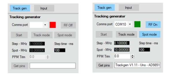
Clicking the **Get pins** button will display the ports the Arduino is currently using to control the DDS device. The ports used may be changed using the **Options** dialogue box, available on the top panel. The ports are displayed as **R:n D:n C:n U:n and S:n**, where **R** is the **Reset** pin, **D** is the **Data** pin, **C** is the **Clock** pin, **U** is the **Update** pin and **S** is the sync output port.
