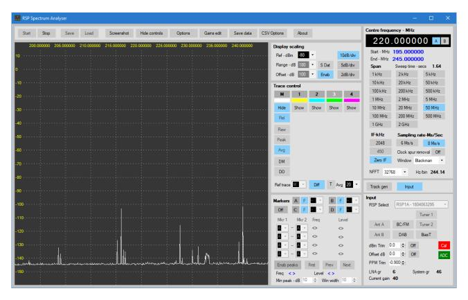
The  $(\mathbf{M})$ ain trace has been used as the reference trace and is placed in average mode. Once the trace had settled, differential mode is enabled. The trace is locked. This trace may then be hidden if required.
