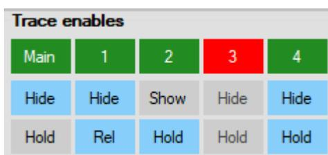
The trace enables panel controls the enabling, displaying and holding of each trace. There are five available traces. The Main trace has the same properties as any of the other traces.
