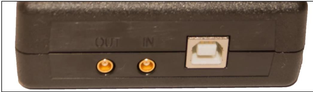
The connection itself is made using an MCX interface and so a suitable cable will be required. The picture below shows an MCX to MCX cable suitable for connecting multiple devices in a master-slave arrangement.
