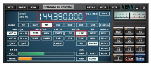
\* Launch SDRuno and select the frequency. The Mode in SDRuno is FM/NFM with the filter set at 12k.
