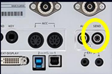
*This control signal must connect to GND during TX*
