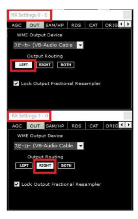
This completes the setup on SDRuno side. Please click each Play! Button. The demodulated signal from ANT 1 is supplied to the L channel of VBA and the signal from ANT 2 is supplied to the R channel. Next, we process these signals on Linrad.
