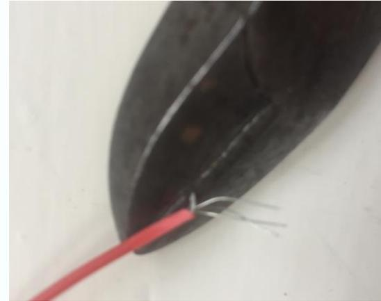
To get started, just strip away the plastic coating from the end of the wire and insert 2 or 3 strands into the centre hole of the coax socket on the RSP1A, taking care not to short against the outer of the coax socket.
