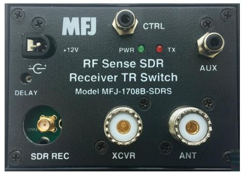
The "B" series offers better isolation, achieved by additional relay isolation, and is specified up to 450MHz. An internal hybrid splitter reduces the antenna loading effect and provides isolation between the rig's input and the SDR input. A TX LED on the front panel provides visual confirmation of correct operation when the transmitter is keyed.
