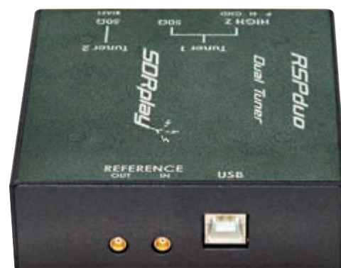
PHOTO 2: The rear panel carries the USB connector and 24MHz reference in and out sockets.
