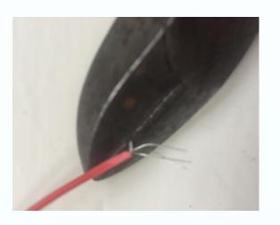
To get started, just strip away the plastic coating from the end of the wire and insert 2 or 3 strands into the centre hole of the coax socket on the RSP1A, taking care not to short against the outer of the coax socket.
