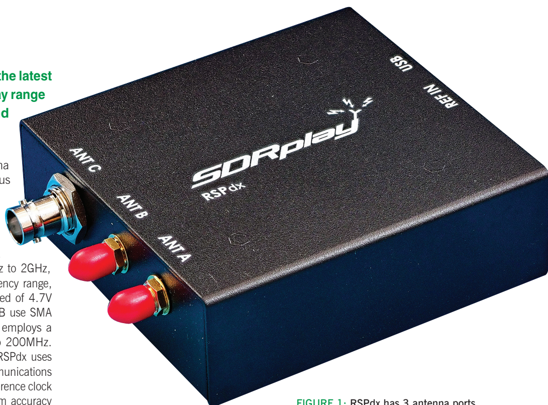
FIGURE 1: RSPdx has 3 antenna ports.
