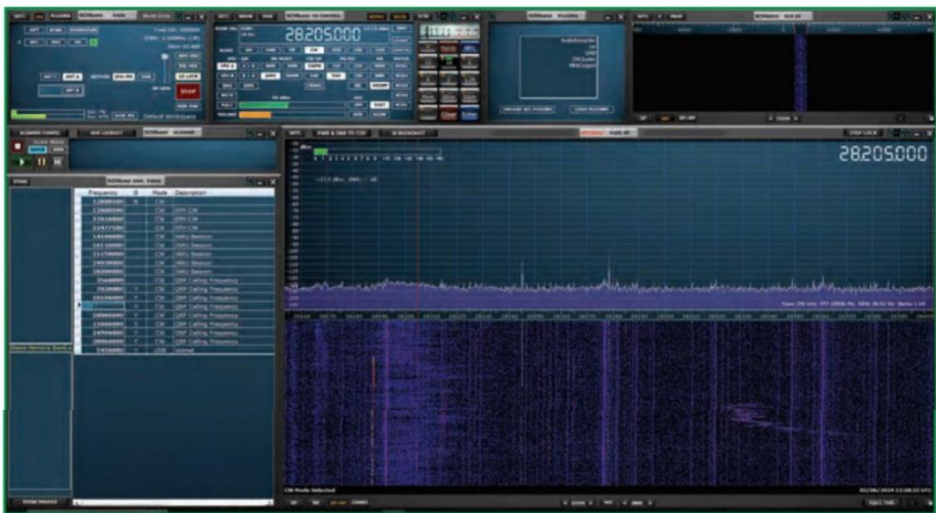
FIGURE 2: A screen grab of SDRplay monitoring the 10m beacon band.
